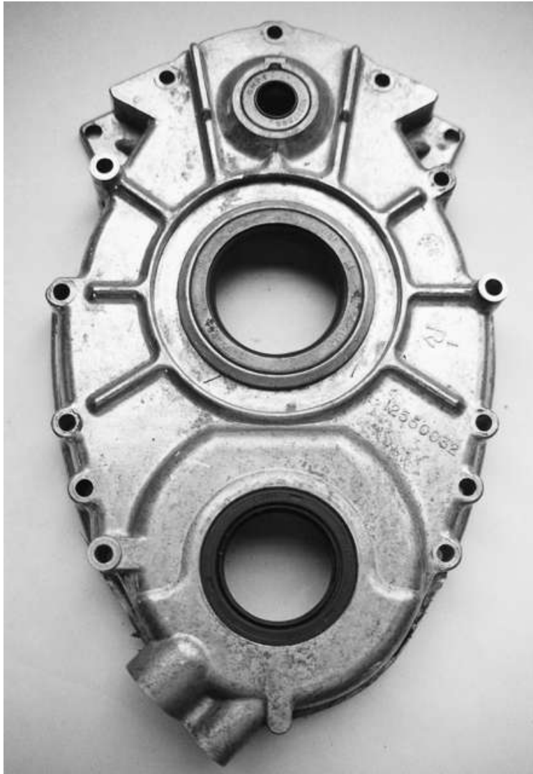
The OBD II-style case has a mounting boss for the crank sensor at the bottom of the casting.
