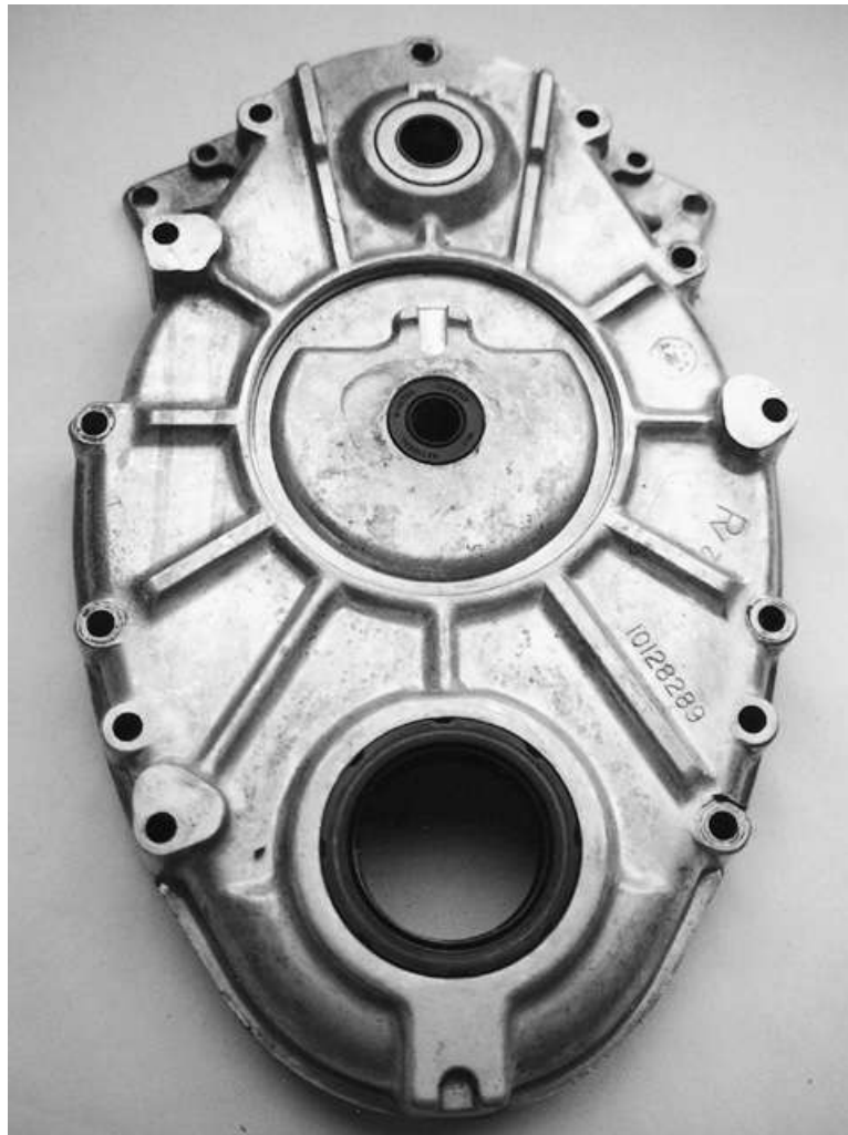
A first-generation timing cover. Note the small hole in the center to drive the distributor.
