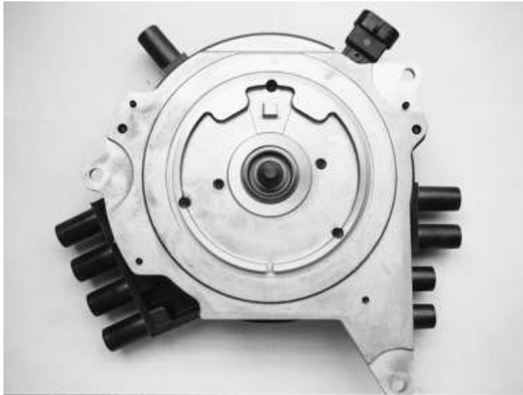
This is an old-style design. Note the small drive mechanism in the center of the distributor.
