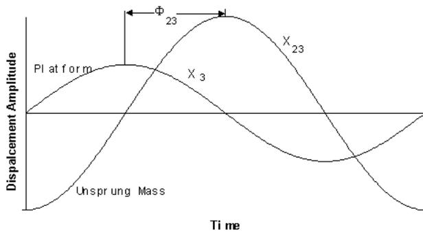
Figure 2. Explanation of Phase Angle
