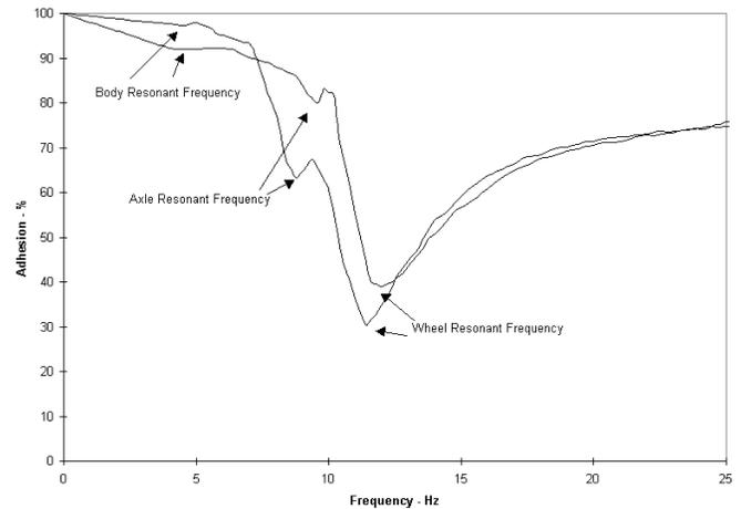
Figure 3. Adhesion vs. Frequency C1500 100% Damper vs. 10% Damper
